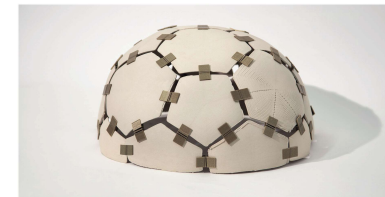
Abb.3: Lightweight dome for a publication at IASS. Double-curved elements are shaped through the shrinkage of a clay layer bonded to a corresponding flat cork layer by paste-based extrusion, 2022, © Shapelab/IAM, TU Graz
